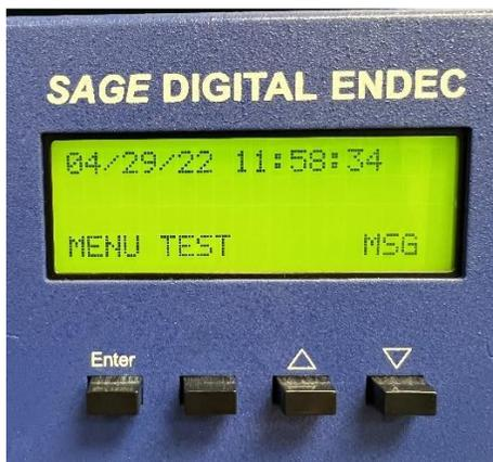
**Figure 3. Endec Front Panel**
